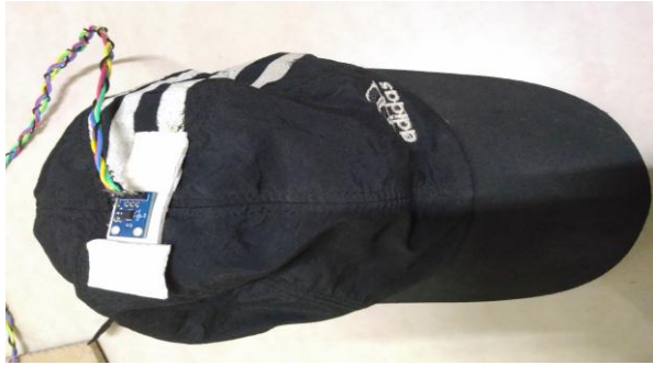
Fig.4: Accelerometer to recognize the head movements
